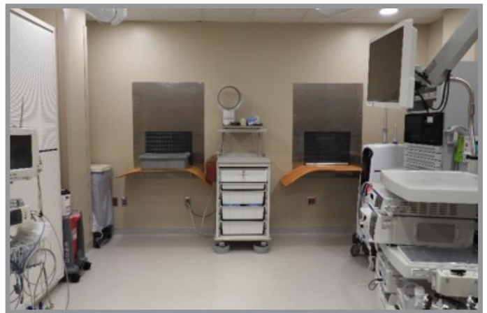
New endoscopy suite equipped with a dirty scope depository and a sterile scope receiving area.
